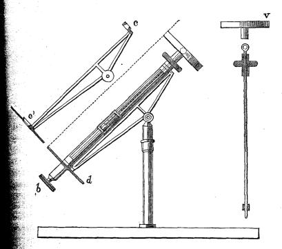
The vessel V is very thin, of silver or plated metal: one determetre in diameter, and 14 or 15 millimetres high; it contains about 100 grammes of water. The stopper which fixes the thermometer to the vessel is fitted to a metal tube which is supported at its extremities by two collets c, c', in which it plays freely; so that on turning the button b, the whole apparatus turns round the axis of the thermometer, and the water of the vessel is incessantly agitated in order that the temperature may
