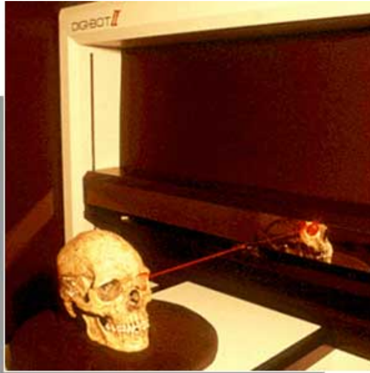
An online skull representation is created from a Quicktime movie of a rotating human cranium by analyzing an actual cranium with a surface scanner, which rotates a specimen on a turntable while using a laser to capture its topography.
